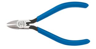
These Electronics Pliers have a tapered nose for easy working in confined areas and close tip cutting. The short jaws have beveled edges for semiflush cutting of wire. The induction hardened cutting knives and hot-riveted joint ensure smooth action and long life. Forged of custom, US-made tool steel for maximum durability.
