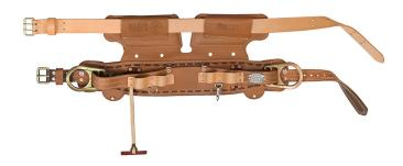
As the title reads, this belt was designed to save a lineman's back. Leather construction is used throughout, including tool loops, tape thong, pocket tabs and cushioning material. Long-lasting 1-1/2" (38 mm) wide double-riveted leather tool loops keep your tools in place. The belt includes four suspender rings, tape thong, two-way knife snap, and glove-bag ring. Forged circle D-rings have corrosion-resistant finish and are proof-loaded to meet OSHA requirements.
