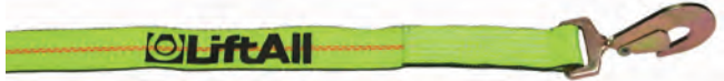
Crossover Strap - Twisted Snap Hook WLL - 3,300 lbs. Use 7 ft. on Weld-Built® Wheel Lifts Length 7 ft. - ATS7T Length 25 ft. - ATS25T Length 28 ft. - ATS28T
