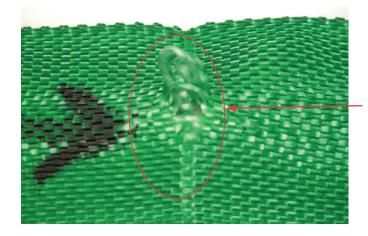
THE DAMAGE: Holes/Snags/Pulls exposing internal core yarns.
