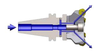
**B.** Modified Shell Mill holder to supply coolant through the sides. Please contact us for more information.
