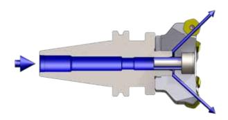
**A.** With coolant slotted bolt (grooves along the bolt): coolant applied through body of the shell mill.
