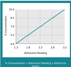
Coolant Refractometer Factor % Brix = 3.1
