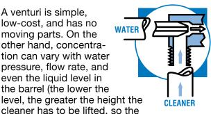
cleaner solution can get more lean). And, if the viscosity of your cleaner is affected by temperature, a cold barrel can give you a leaner solution than if the cleaner were at room temperature. (So, if you store your drums outside in cold weather, it's a good idea to bring them inside for a day or two to warm up before you need to use them.) Don't get us wrong, venturi mixers are still a good choice to mix cleaners accurately for a lot of applications.
