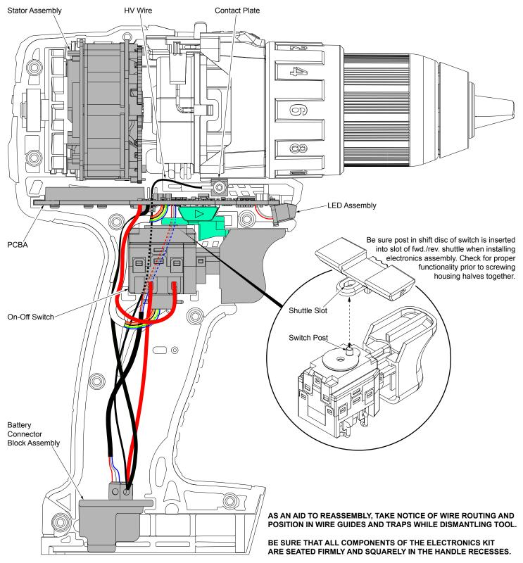
AVOID PINCHED WIRES, BE SURE THAT ALL WIRES AND SLEEVES ARE PRESSED COMPLETELY DOWN IN WIRE GUIDES AND TRAPS.
