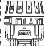
**NOTE:** The number selected on the torque selector collar has no effect on operation of the drill in drilling mode.
