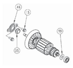
**31-50-1752 Motor Housing Kit** incorporates changes to the shielding of the armature pinion and commutator ball bearings along with the retaining of the pinion ball bearing into the gearcase assembly of 7"/ 9" 15Amp Sander / Grinders – 6080-20, 6081-20, 6082-20, 6086-20, 6088-20 and 6089-20.
