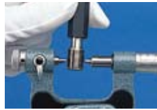
116-101 with matching optional interchangeable anvil and spindle-tip fitted ready for measurement
