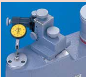
Calibrating test indicator
