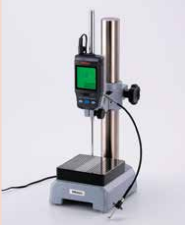
Application example using Digimatic Indicator ID-H.
