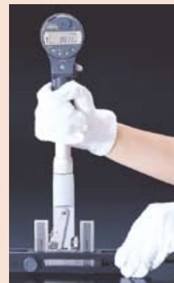
Setting the Bore Gage to a master value using a gauge block set
