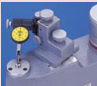
Calibrating test indicator
