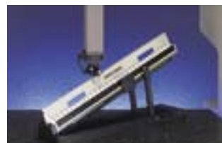
CMM calibration with Check Master No. 515-742
