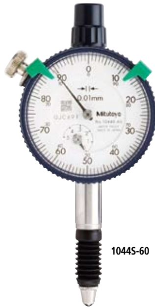
Graduation: 0.01mm, Measuring range: 5mm 1044S-60 Waterproof
