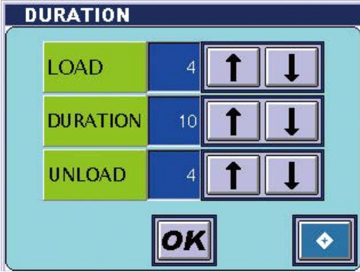
In addition to the test force duration time, you can specify loading and unloading testing actions.
