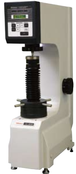
HR-430MS 963-241 Dual type (Rockwell/ Rockwell superficial combined use) hardness testing machine Economy type, but supports dial switching power steering and support of all test standards and equipped with automatic brake handle auto start feature. Motor drive controls loading sequence.
