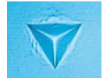
Indentation by triangular pyramid indenter
