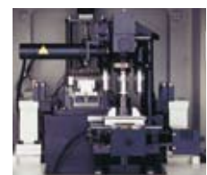
Interior of the automatic multi-point measurement device with the XY automatic stage
