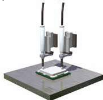
③ Chip parallelism measurement
