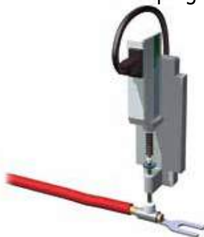
5 Measurement of crimping height
