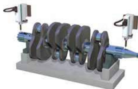
6 Workpiece height detection
