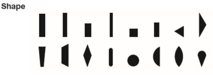
• Area to be filed will determine specific cross-section (round, square, flat, etc.) to be used.
