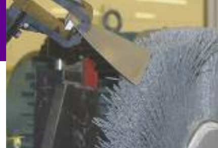
Deburring the tip of a turbine blade.
