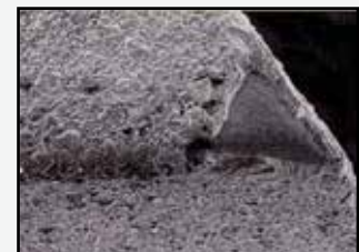
Diamond Delamination (Note: Large Grain Size)
