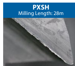
Wear Condition of the Cutting Edge
