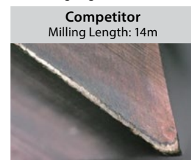
Wear Condition of the Cutting Edge
