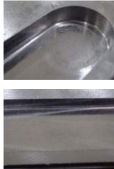
Plunging to Horizontal Milling
