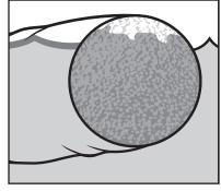
When completely saturated, the boom will 'bob' just below the water's surface. (Boom must now be replaced). Fluid stays absorbed, and retrieval is easy.
