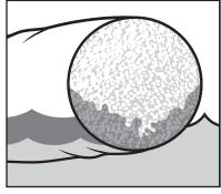
Put in spill on water. Boom begins to absorb as soon as it's in place. No water soaks in — only petroleum products.
