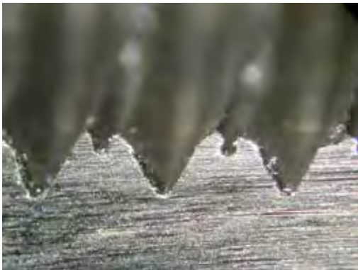
Section of thread obtained by forming tap on steel C45
