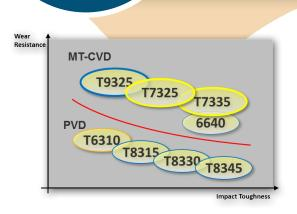
The T7325 grade is available on both positive and negative inserts with chip-breakers suited for machining M and S-group materials in roughing through finishing operations.
