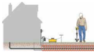
Direct connect to utility lines
