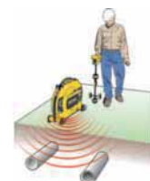
Induce a signal to locate utilities
