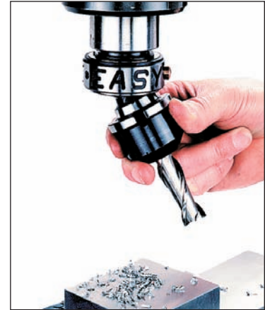
4. Inserting endmill holder and endmill for next operation.
