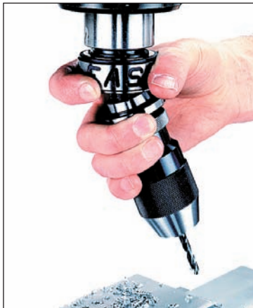
3. Removing drill chuck holder with one hand.
