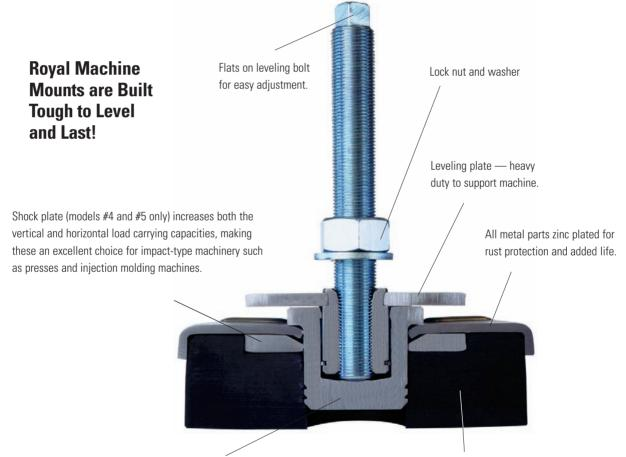
Heavy-duty support cup is machined from a solid steel bar for strength. Other brands rely on a thin drawn cup which often fails by fatigue. Note the increased thickness of the lip and bottom sections.
