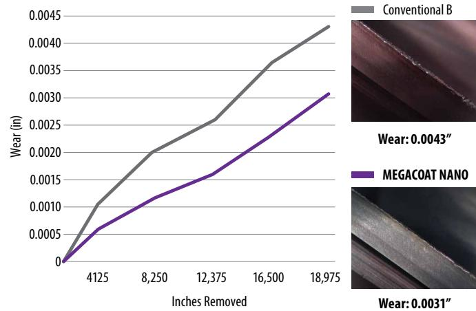
Cutting Conditions: 1/2" Dia. Tool, Speed = 6,066 rpm (794 sfm), Feed = 145 ipm
