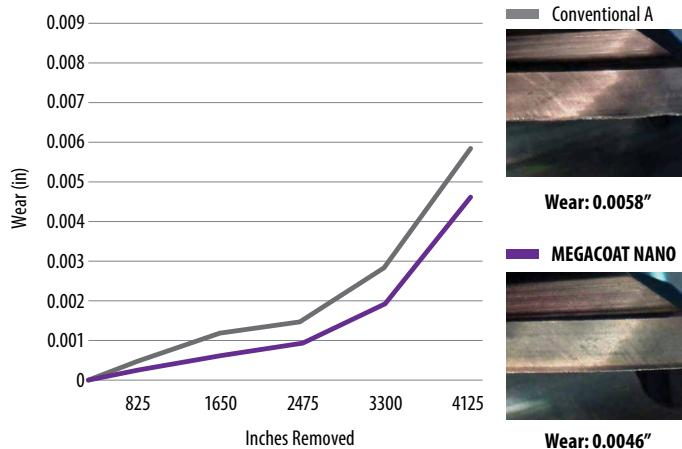
Cutting Conditions: 1/2" Dia. Tool, Speed = 4,332 rpm (567 sfm), Feed = 76 ipm
