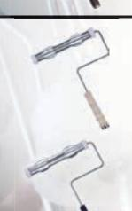
Heavy-duty 8mm (5/16") chrome-plated steel shank, reduces bending when using with an extension pole. Two tension bends on five wire cage assembly to prevent refill creeping. Available in both natural hardwood and injection-moulded plastic handles with metal insert or grommet for extra strength. Threaded for use with extension poles.
