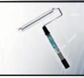
Sturdy 6.4mm (1/4") galvanized steel shank. Two tension bends on five wire cage assembly to prevent refill creeping. Available in two unique Simms comfort design injection-moulded plastic handle designs. Threaded for use with extension poles.
