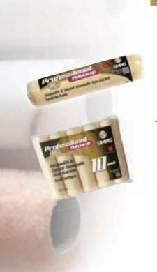
**Polylamb®**. High density, knitted polyester and nylon fabric blend. High paint carrying capacity. Ideal for applications where coverage is required such as drywall priming, painting on particle board, plywood, masonry surfaces and other exterior jobs. 6mm pile for all flat, low sheen and semi-gloss latex paints or flat and low sheen oil paints. 10mm for flat and low sheen paints. 13mm to 31mm piles for all flat paints. Solvent resistant polypropylene core.
