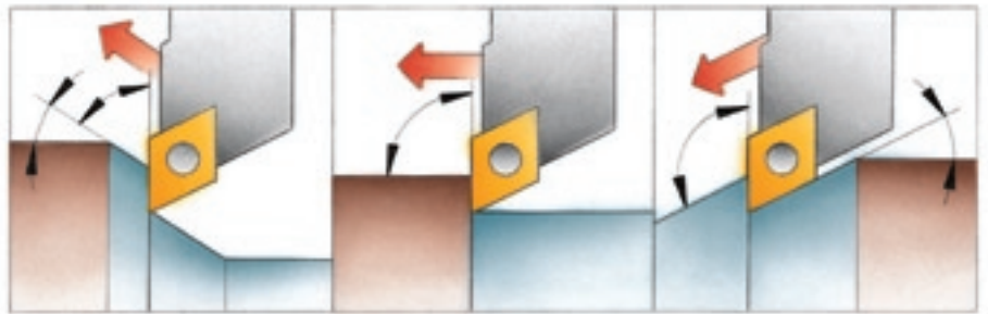
The effective entering angle ( \kappa_1 ) should also be considered for satisfactory machining when the operation involves copying or profiling. The maximum in-copying angle ( \beta ) is recommended for each tool type and treated more thoroughly in the part on Copying.
