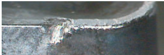
Competitor grade after 3.5 min in cut.
