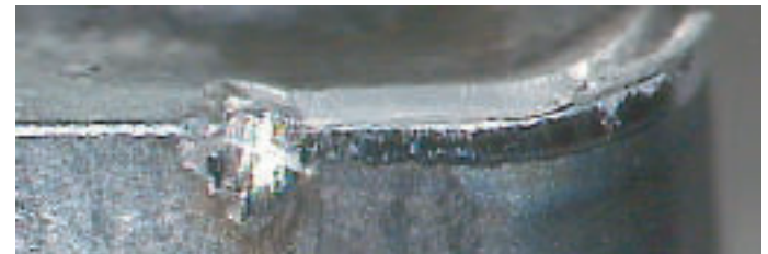
New grade GC1105 after 5 min in cut.
