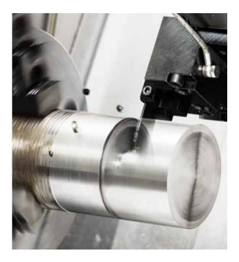
Tool overhang is one of the main factors to always minimize in any machining operation but in parting off large-diameter bars and when having to have extended reach, long overhang is unavoidable. This leaves it up to the tool to compensate for the inherent instability of the operation and to have the capability to ensure a safe, satisfactory operation that is also competitive. A parting-off tool-system dedicated for depth and overhang is a necessity today.
