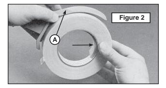
Pull 3 to 4 inches [80 to 100mm] of tape from roll while ensuring that the inner tape edge is folding over by applying tension to the roll brake. Pull on lead end tab to thread tape through and over roll spring (B) (see arrow Figure 3).
