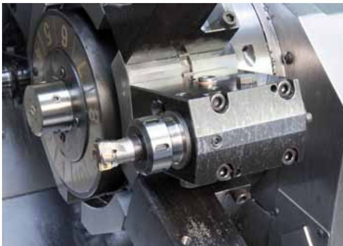
Multi-task machine, rotating turret with ER spindle, equipped with an ER to Combimaster adapter and a Combimaster milling cutter.
