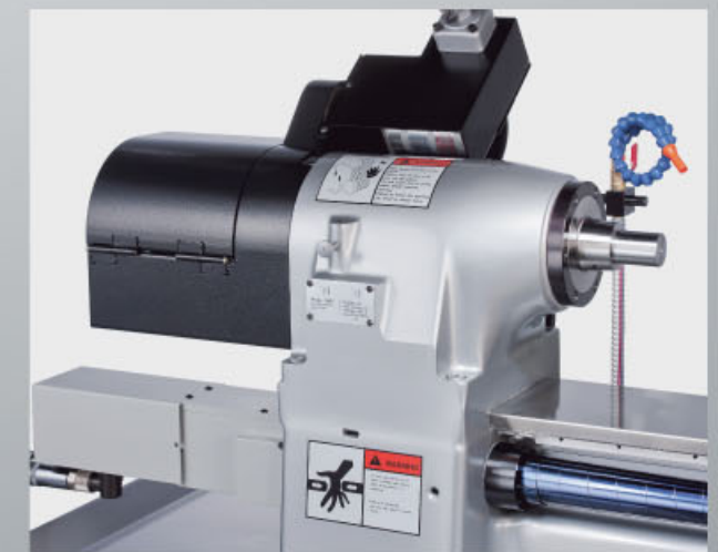
Air operated collet closure (with foot switch) is provided as a standard accessory for quick and easy release of a workpiece. A pull-down style chip guard protects the operator from flying chips. Full length splash guard is mounted at the back to contain coolant splashing and flying chips.
