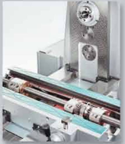
Double box ways on saddle, also showing power feed table driving mechanism.
