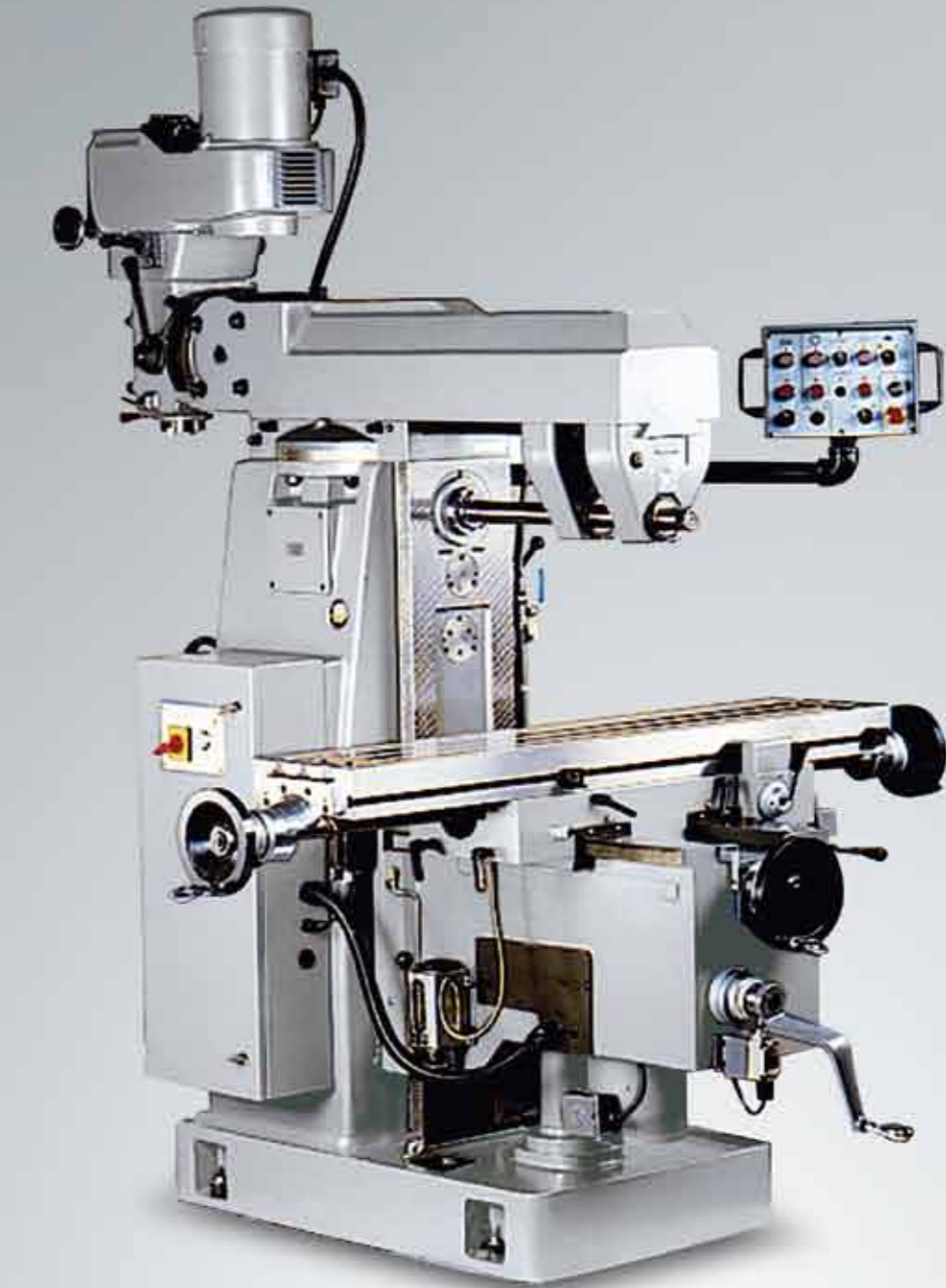
Double box ways on saddle, also showing power feed table driving mechanism.
