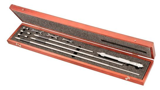
Using the tool: Remove the eight-inch-long micrometer measuring head assembly and if the required distance is longer than 9 inches, loosen the knurled collet on the end opposite the micrometer section. Once loosened remove the rod and consult the table below for combinations of rod/spacer(s) required to attain the desired length.
