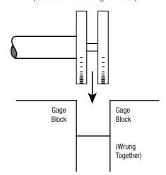
In each case the micrometer sleeve is set to agree with the setting master to eliminate any play affecting the reading.
