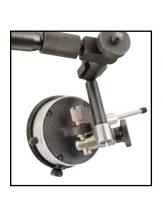
Choice of two ways to fasten the indicator to the end of the Flex-O-Post
