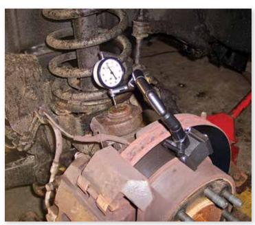
S898Z-2 configured with the magnetic base to secure the measuring setup in place
