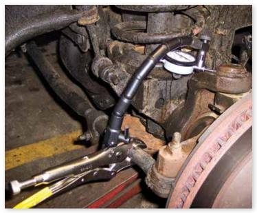
S898Z-1 configured with the pliers to secure the measuring setup in place
