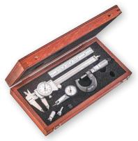
This basic mechanical tool kit includes a one inch micrometer, six inch steel rule, dial slide caliper, and test indicator. Set comes in an attractive wooden case.
