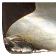
ER chuck wear detail
