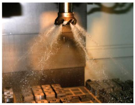
CoolBLAST arbor screw provides coolant path.
