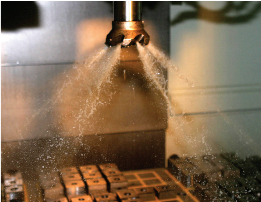
CoolBLAST arbor screw provides coolant path.
