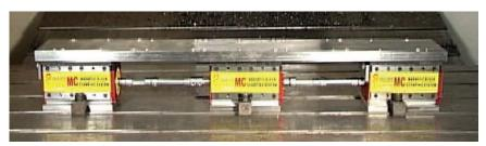
Switch-connect ECB vises to turn ON/OFF simultaneously
