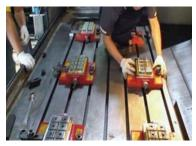
Position the chucks on the machine bed.
