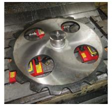
Large tooth sprocket being machined
