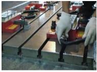
Connect the control cables to chucks and control
