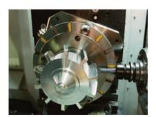
Off-axis rotation on horizontal mill
