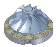
5-axis turbine blade machining
