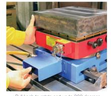
Pull knob to rotate part up to 360 degrees
