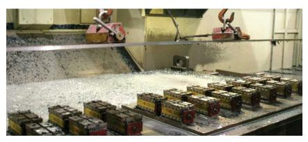
...or use multiple ECB vises positioned as needed to hold large parts.
