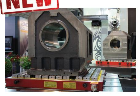
Our 70MM pole chucks provide the increased holding power needed for large workpieces, thick plates, blocks and molds. Great choice for drilling, milling, and boring operations on vertical or horizontal mills. They easily integrate with pallet changing and tombstone systems.
