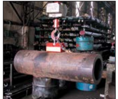
Beveled bottom surface lifts round stock.
