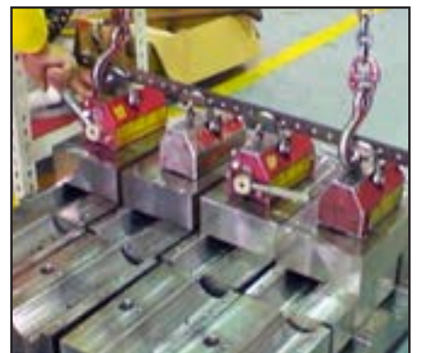
Use spreaderbars to gang stock in one operation
