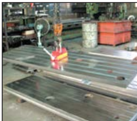
Locate magnet at balance point for lifting.
