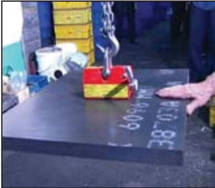
3.5 X Safety Factor above rated load capacity
