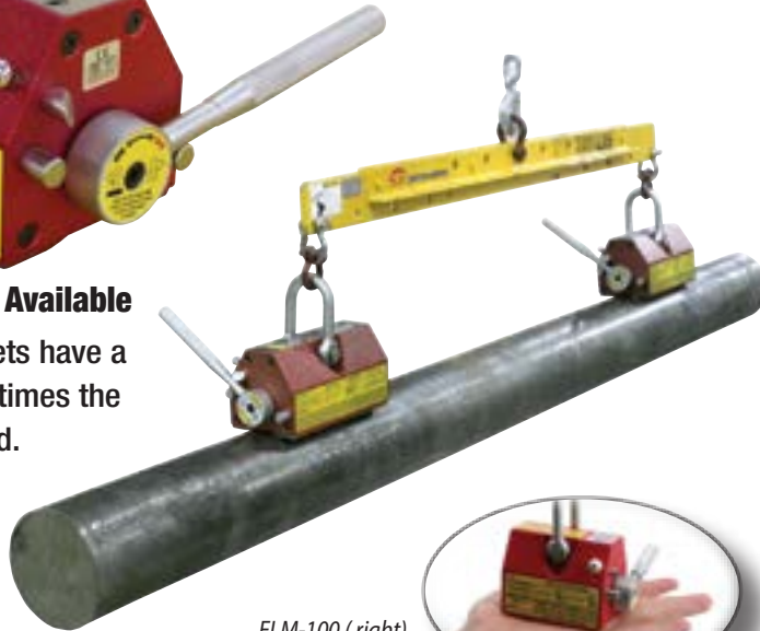
ELM-100 (right) weighs 5.5 lbs. and lifts 220 lbs.
