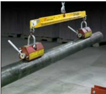
Use spreader bars for long, difficult round stock
