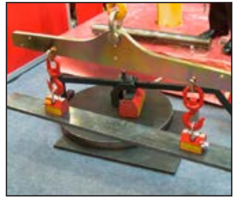
Spreader bars are used for long or very heavy loads.
