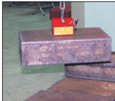
Center magnet on most workpieces to lift.
