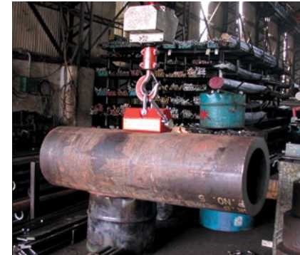
Beveled bottom surface lifts round stock.
