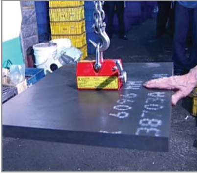
3.5 X Safety Factor above rated load capacity
