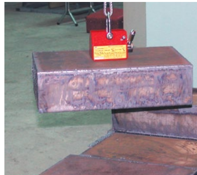
Center magnet on most workpieces to lift.
