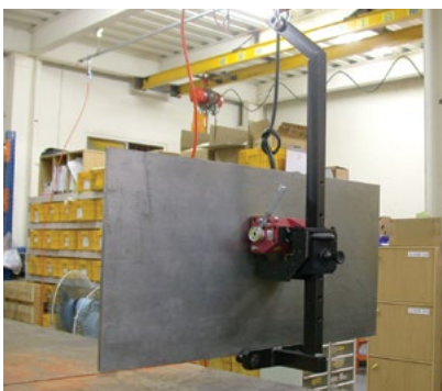
Vertical Lifters can be operated by one person.
