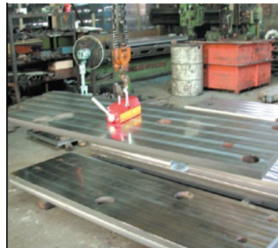
Locate magnet at balance point for lifting.
