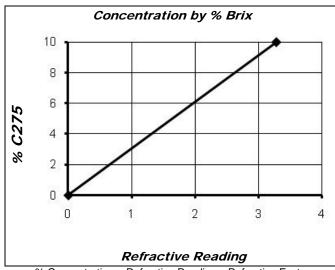
% Concentration = Refractive Reading x Refractive Factor Coolant Refractometer Factor % Brix = 3.1
