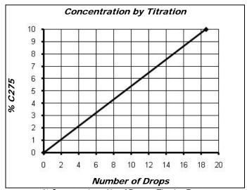
% Concentration = No. of Drops x Titration Factor Titration Factor = 0.540
