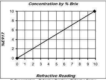
% Concentration = Refractive Reading x Refractive Factor Coolant Refractometer Factor % Brix = 1.0
